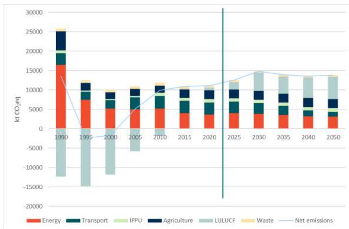
Figure 2-8 Total amount of GHG emissions of Latvia (until 2020) and projection (for 2025-2050) under the scenario “with current measures” (1990-2050) 51
