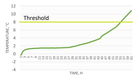
Excellent performance ensuring temperature from -2°C to +8°C for 42 hrs with test chamber temperature of +30°C and 55 hrs with test chamber temperature of +22°C.
