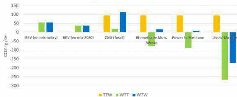
WTW emissions comparison c-segm vehicle - WLTP - Renewable gas options
