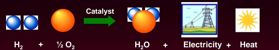
Fuel cells combine hydrogen and oxygen electrochemically to produce electricity
